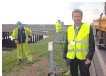
Graham Chappell looks on as engineers perform a "push-pull" test on barrier posts prior to the installation of barriers on the sixteen foot road
